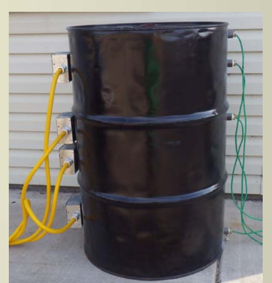
Test tank with four 3kW water heating elements with yellow cords, and four temperature sensors with green cords.
