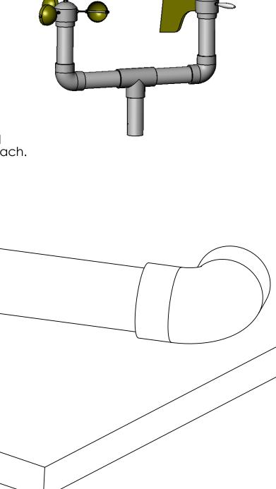
Included Materials: 2 x Right Angle Fittings 1 x Tee fitting 2 x 6" PVC pipe 1 x 5" PVC pipe with wiring
