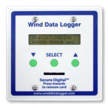
The Wind Data Logger records directly to a Secure Digital (SD<sup>™</sup>) card to provide convenient data downloads. The included SD<sup>™</sup> card will store many years of data. The default logging interval for recording data to the memory card is 60 seconds, which is suitable for most applications; however the logging interval can range from 10 to 60,000 seconds. For your convenience, a new file is created and saved to the card for each day the logger is in use.
