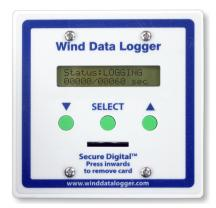
The Wind Data Logger records directly to a Secure Digital (SD™) card to provide convenient data downloads. The included SD™ card will store many years of data. The default logging interval for recording data to the memory card is 60 seconds; however the logging interval can range from 10 to 60,000 seconds. For your convenience, a new file is created and saved to the card for each day the logger is in use.
